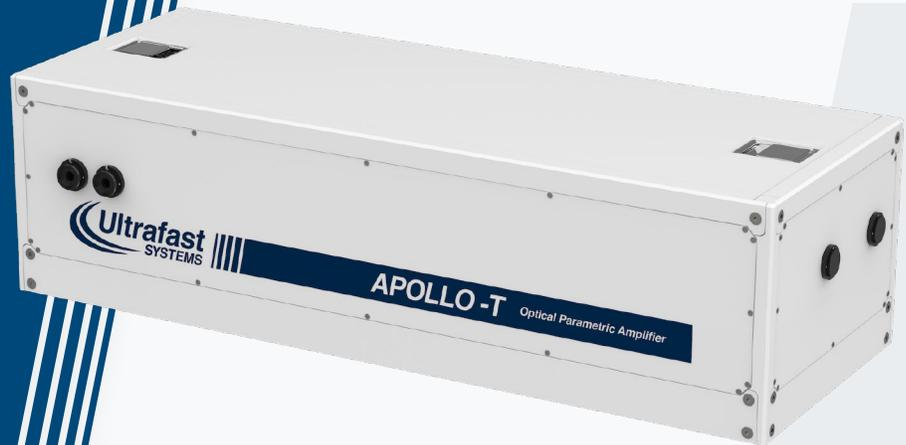
The **APOLLO-T** OPA is designed to extend the tuning range of a kHz Ti:Sapphire amplifier from the UV to the Mid-IR. It is optimized to work with Ultrafast Systems' [spectrometers](#). High stability and high efficiency are achieved through two step amplification of a white-light supercontinuum, and nonlinear crystal tuning, optical delay compensation, and wavelength separation is fully computer controlled.
