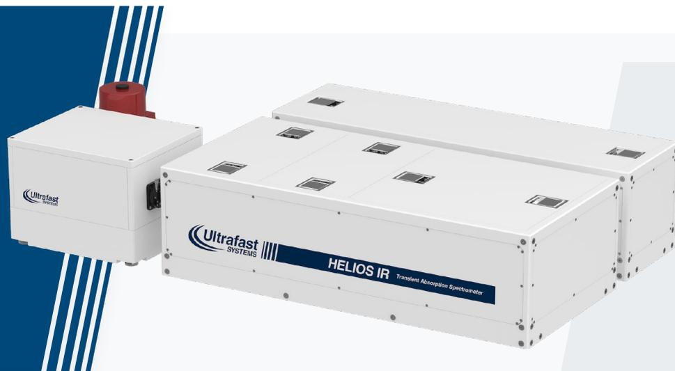
**HELIOS IR** is a broadband mid-infrared femtosecond Transient Absorption Spectrometer. A complete turn-key system, HELIOS IR can measure photoinduced absorbance changes across a broad (2-13  $\mu\text{m}$ ) spectral range with femtosecond time resolution over an 8 ns time window. At any time, the HELIOS IR time window can be extended to sub-milliseconds with an EOS IR add-on.
